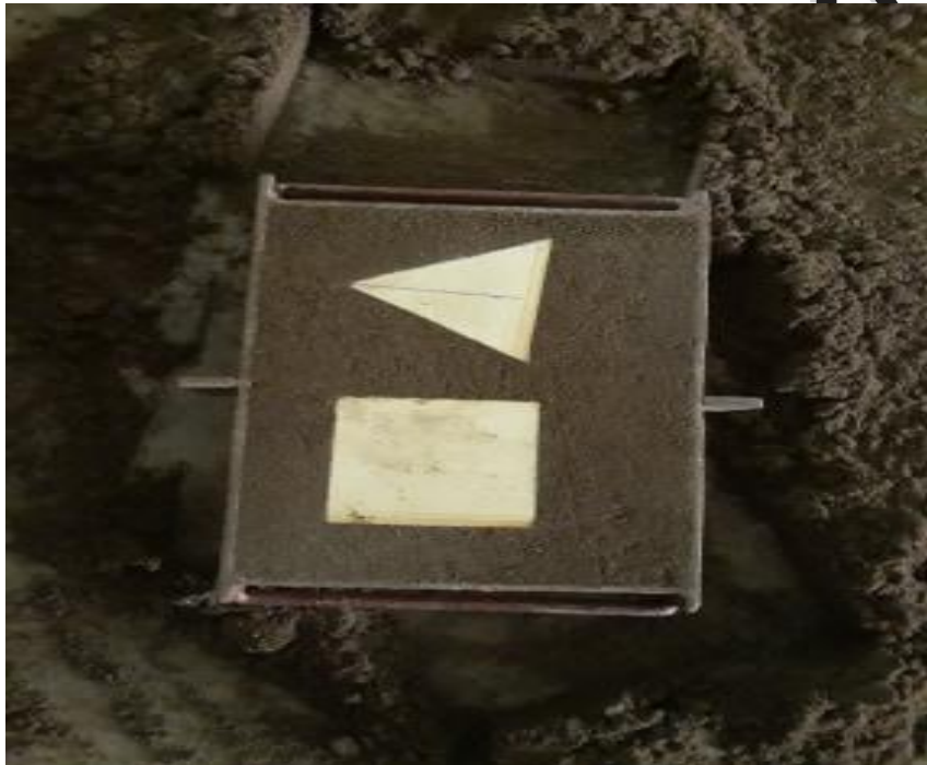
Figure 2 Developed the Mold for Casting
